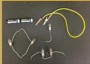
Figure 1. Components of the physical setup, including batteries, alligator clips, and a single bulb in addition to bulbs wired in both parallel and series.
