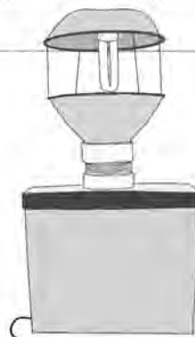
A fully assembled capture-mark-recapture trap (CMRT).
