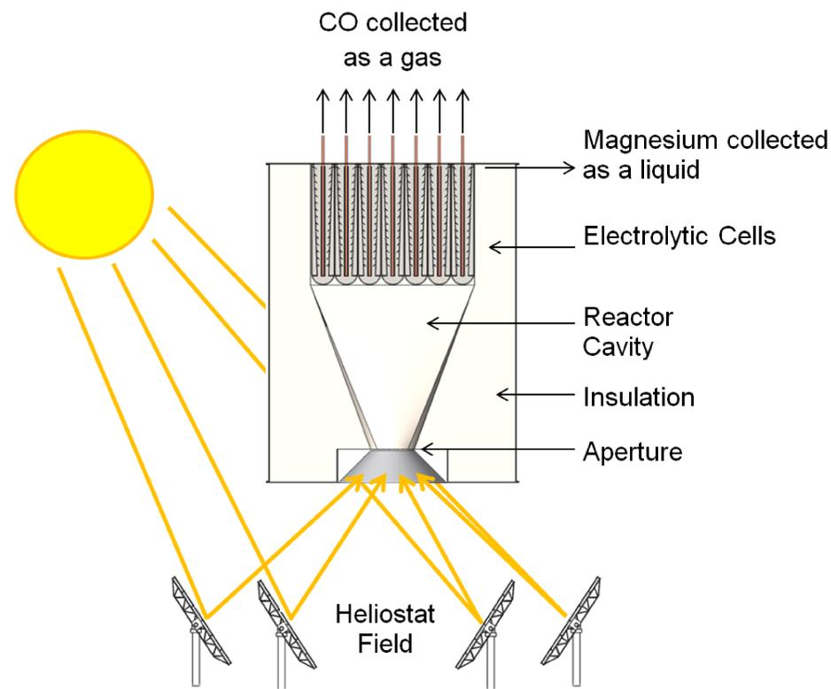
Industrial scaled process for Mg production using solar thermal electrolysis
