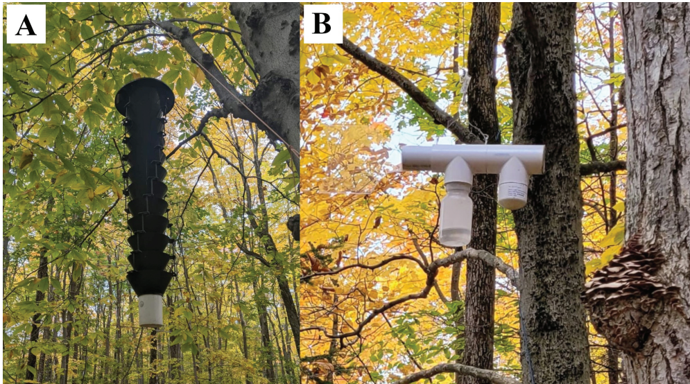
Figure 2. Two trap types used in the oak wilt vector surveys in Quebec. A) Lindgren funnel trap, B) Wind-oriented pipe trap.
