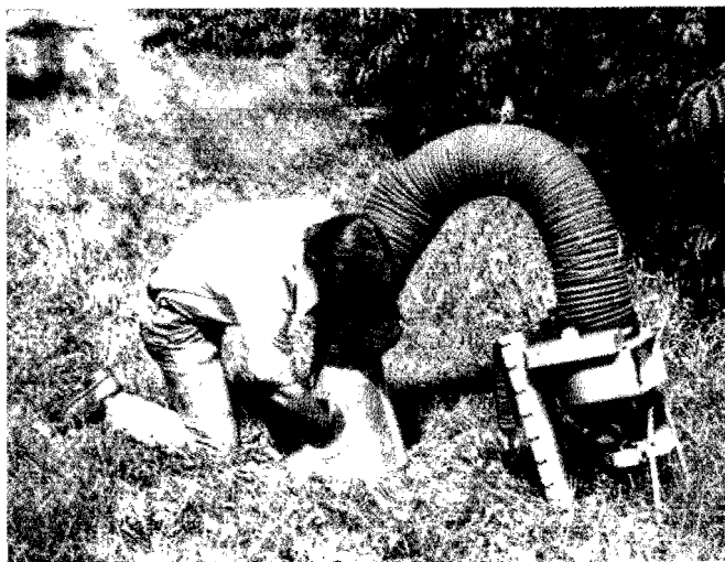
Fig. 1. Ground sampling device with attached D-vac® showing method of operation.
