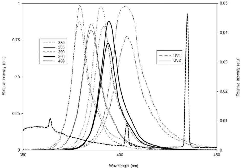
**Figure 2.** Peaks of light intensity within the 350–450nm range for the 10 LED (primary axis) and 2 fluorescent UV (secondary axis) bulbs tested. Intensity is in arbitrary units (a.u.), because bulbs were tested to confirm their primary wavelengths only. Thus, the spectrophotometer was not calibrated for absolute intensity, precluding any meaningful comparison of intensity between bulbs.
