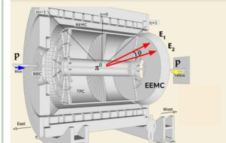
Figure 2: A digital model of STAR. The EEMC is shown to the right. Both proton beams are shown.
