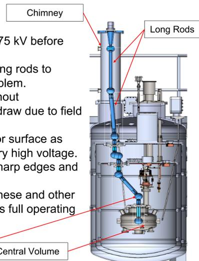
Figure 7: HSHV system showing the HV chain (blue) for transferring 200 kV from room temperature to the central volume ( $<2 \text{ K}$ ).
