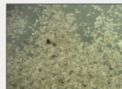
Roto Powder Sized Between 0.20mm to 0.80 mm
