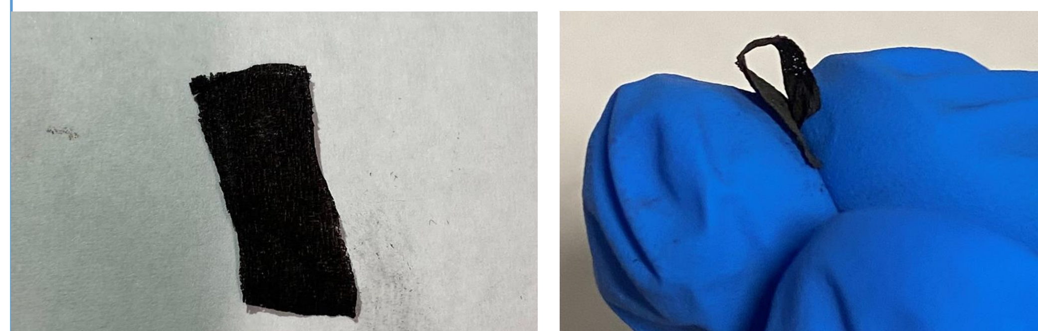
Figure 3 Flexible rGO film after reduction in tube furnace.
