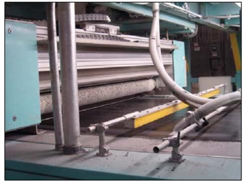
Next, the top fibers are sheered, separated, and formed into new threads. All polymer-based nylon fibers are extracted from the backing which end product is then used at other businesses to produce such parts as vehicle dashboards. The residue is shaped into small, round balls or crumbs, known as “Cool Blue Food™” – harmless to the human system as the new substance lacks toxins, metals, and nonorganic flame retardants.
