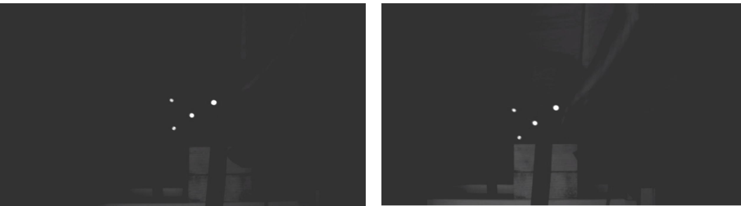
FIG. 5: A pair of images captured by the stereo cameras at approximately the same time, in front of the coil discussed above. The bright spots are reflective markers attached to the fluxgate magnetometer probe. The data shown above was collected using a single attached marker; these images were recorded to develop another tracking method.
