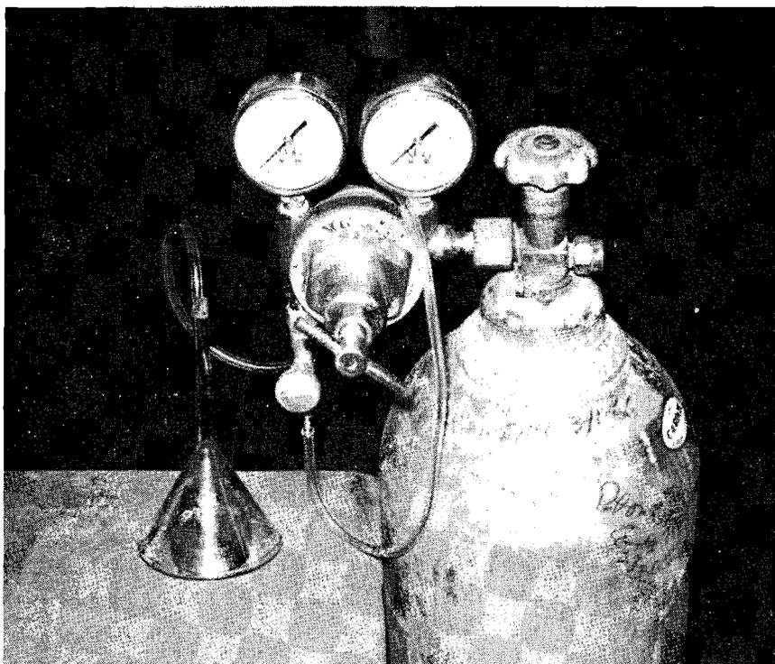
Fig. 8. CO<sub>2</sub> technique with culture jar in place.
