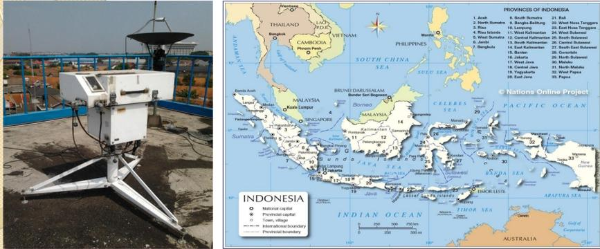
Fig. 1. Brewer spectrophotometer (left) used for the measurement of total ozone,  $\text{NO}_2$  and  $\text{SO}_2$  columns over Bandung, Indonesia (right) (Source: Nations online project, 2012). It was placed on the top roof of the fourth floor of LAPAN office
