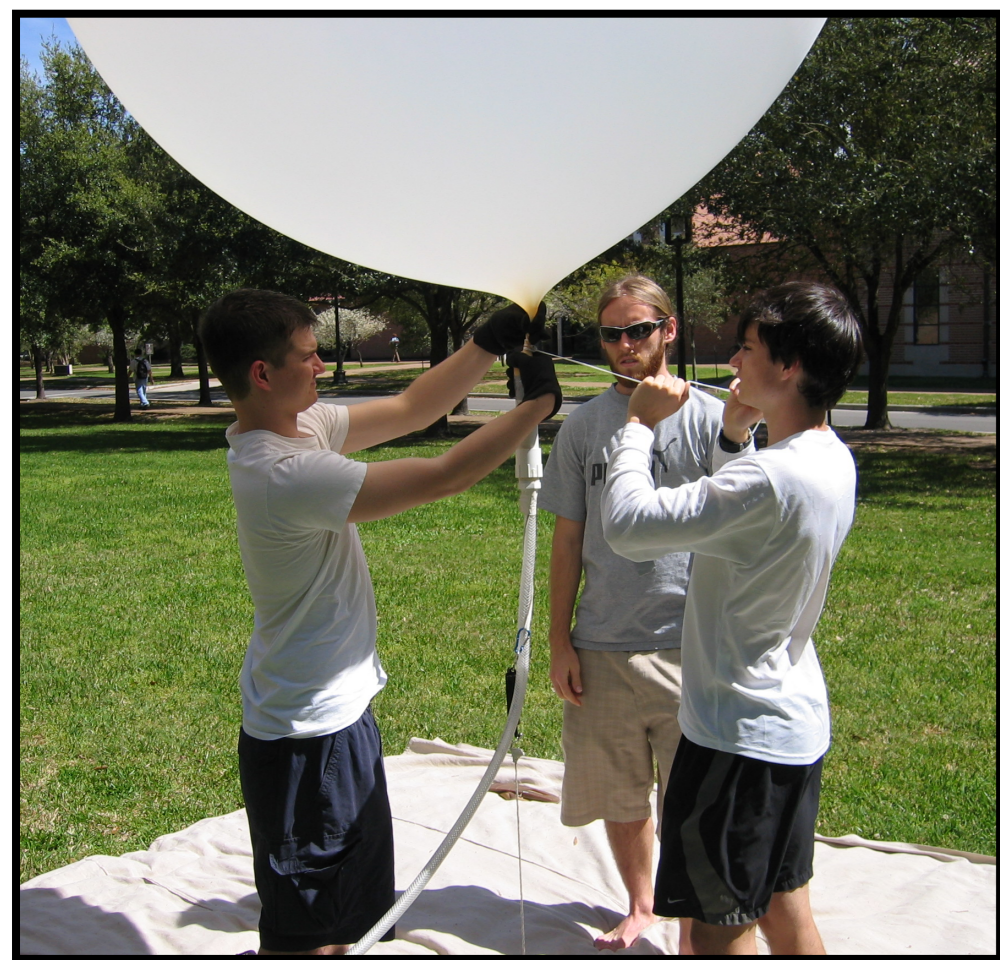
Figure 1. Rice Univ. students prepare an ozonesonde for launch during the Summer 2005.
